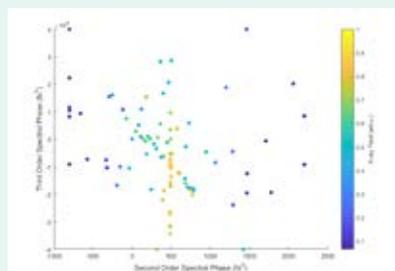
Figure 1: Every trial solution attempted by the genetic algorithm across all generations, with the colour representing the x-ray yield of each trial solution
