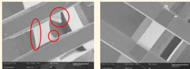
Left: SEM Image of aluminium strip produced by removal of a plastic support layer. Areas of contaminant can be seen circled in red.
