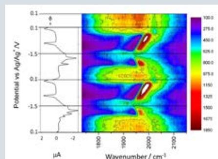
VSFG spectra showing how surface electrochemical events seen by the current-voltage response (left) can be monitored using VSFG spectroscopy (right) where we see new  $\nu(\text{CO})$  bands forming at the potentials of the electrochemical events.
