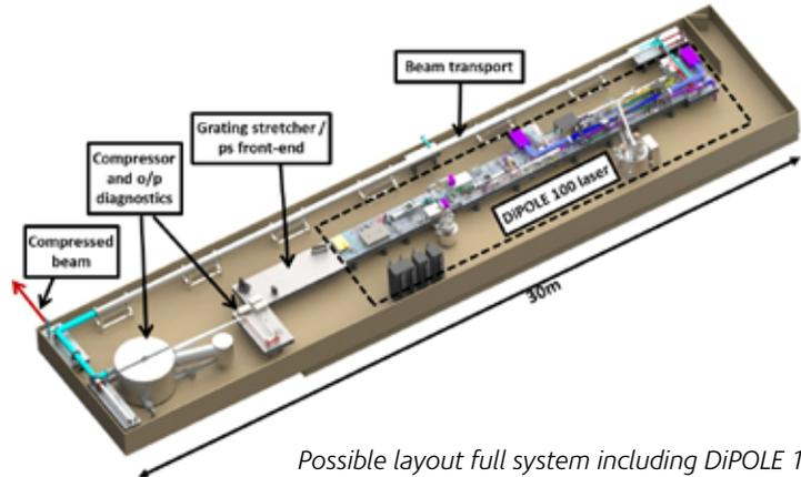
Possible layout full system including DiPOLE 100 laser, front-end with stretcher, compressor, and beam transport
