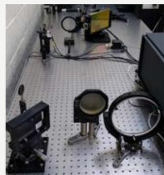
Figure 2: (right) Photograph of initial compressor setup. Beam enters from top right, G1 is located in the bottom-right, G2 top-left and RM1 bottom-left
