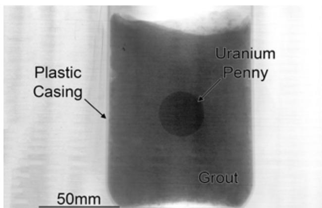
*Radiograph of uranium penny encased in grout obtained using single pulse of a laser-driven x-ray beam.*
