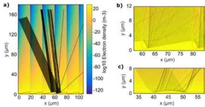
[a] Ray trace of a sawtooth plasma grating structure, demonstrating that the majority of the incident rays are reflected from the grating at a consistent angle, which is different to the incident angle. The red line shows the critical surface of the plasma.
