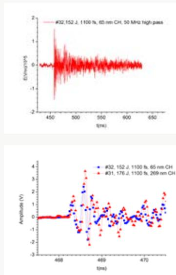
Top figure: The vertical component of the electric field intensity  $E$  as a function of time  $t$ , recorded with a D-dot probe placed just outside of the chamber in a glass window, as obtained after applying 50 MHz high pass filter.
