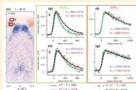
(c) Difference between the ARPES image 80 fs after and 200 fs before optical excitation. (d) - (e) Population dynamics of MoTe<sub>2</sub> integrated at 50 K (blue) and 300 K (red) in the area highlighted in panel (c) by the rectangles. (f) - (g) Comparison between the population dynamics measured at 50 K (blue) and 300 K (red) in WTe<sub>2</sub>. The best fit and the corresponding characteristic time are shown, as well.
