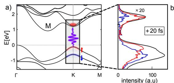
a) DFT calculations of the band structure of bulk WSe<sub>2</sub>. At the K point, the two valence bands are purely spin polarized. The material is excited with 1.5 eV circular polarized light pulse populating the conduction band in the K valleys. The grey shaded area corresponds to the probed area with the spin-resolved detector.
