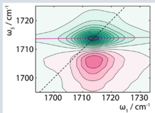
Isotropic 2DIR spectrum for the C–N anti-symmetric stretch vibration of the formamidinium cation in lead iodide perovskite films
