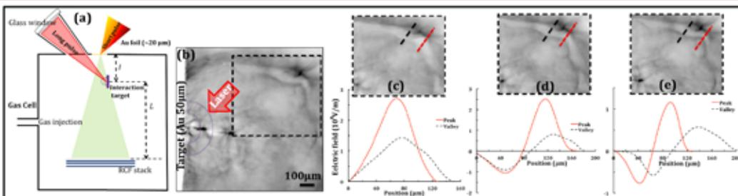
(a) Schematic of the experimental setup (top view). The experimental set up was enclosed in a gas cell, which was placed inside the vacuum chamber. (b) proton radiographs of the interaction of a nanosecond laser pulse (red arrow) with a 50 μm thick gold foil, correspond to time  $(t_0 + 6)$ ps from the start of interaction. The spatial scale shown in the image (b)
