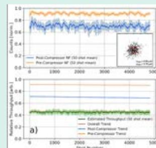
Figure 2: Pre- and post-compressor energy measurements and relative throughput for 4950 laser shots at 5 Hz. The inset shows the beam pointing variation relative to the 20 μm focal spot size.
