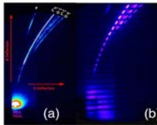
Figure 1 (a) MCP imaged on shot with Andor Neo CCD (false colour) (b) calibration shot using slotted CR-39 through which the carbon passes.
