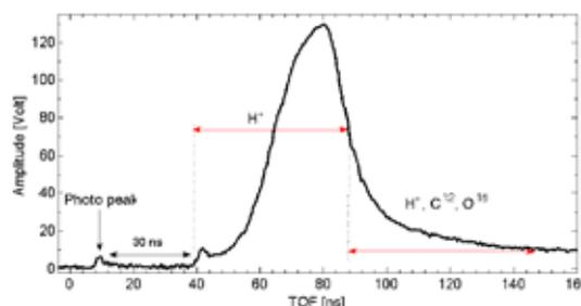
*TOF signal acquired with a 100  $\mu$ m thick diamond detector placed @ 2.35 m downstream from the target.*
