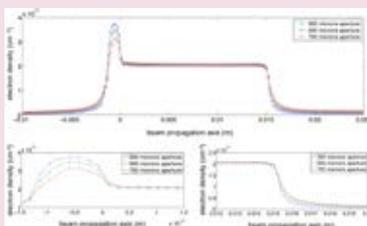
Figure 1: (a) Electron density distribution along the full gas cell, zero is the middle of the separation wall, depending on the aperture diameter; (b) density down-ramp between acceleration and injection stages; (c) density tail at the exit.
