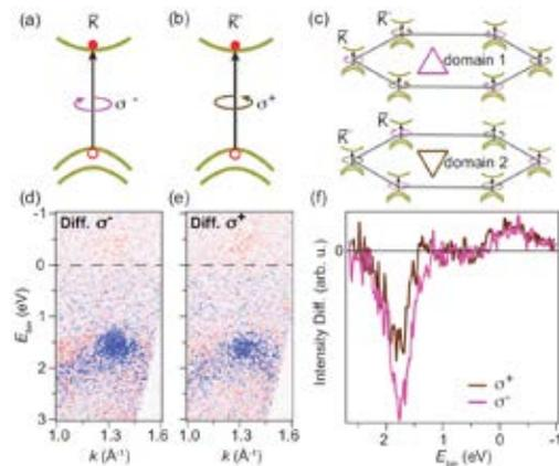
(a),(b) Schematics illustrating the selection rules for transitions from the upper VB to the CBM in the K and K' valleys. (c) BZ orientations and selection rules for the two mirror domains of the SL WS<sub>2</sub>. (d),(e) Difference signal for optical pumping with (d)  $\sigma^-$ - and (e)  $\sigma^+$ -polarization. (f) EDCs of the difference integrated over the VBM and CBM regions for the data in (d) and (e).
