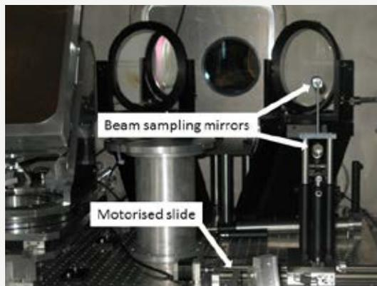
The new beam-sampling setup in the Gemini south compressor
