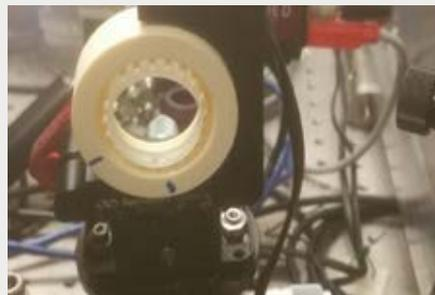
Figure 2 LBO crystal held in place by a laser printed holder which is fixed in a 50 mm mirror holder with electronic actuators for changing the angle of the crystal remotely.
