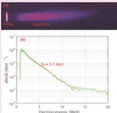
An electron spectrometer has been employed in measuring escaping electrons from laser-solid interactions. Electron spectra have been obtained in different laser pulse conditions. Dependence of escaping electron numbers and temperature on the pulse energy, intensity and duration is shown in this report.
